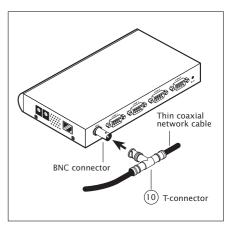
**Note**: If you leave any open end on the T-connector, attach a 50-ohm terminator to this end.
