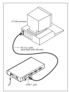
**4-** UM link will automatically detect the terminal as soon as it is connected. Press "+" twice. UM link's built-in terminal program will be invoked and the following main menu will be brought up to the terminal 's screen.
