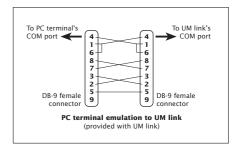
**Note**: You can use one supplied serial cable with a null modem adapter between your PC on terminal enulation mode, and the UM link COM 1 port.
