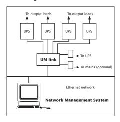
UM link is equipped with built-in SNMP agent software and processing hardware, an Ethernet port, and four communications ports for UPS connections, permitting management of the UPSs from a network manager station using a standard management protocol.
