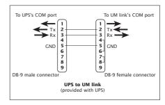
**Note:** UPS reception through pin 2 (Tx), UPS transmission through pin 3 (Rx). You can also use standard 3-wire (2,3,5) straight-through serial cables to connect UPS to your UM link.
