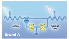
Other conversion topologies have limited isolation from the dangers of utility power, letting raw utility power flow right through the UPS to devices on the output.
