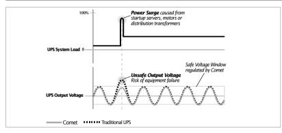
Computer power supplies and distribution transformers draw extreme surge currents when they are powered up. This often causes sags and surges on the UPS output compromising other devices already on UPS power. To eliminate this frustrating phenomenon the Comet UPS was designed to instantaneously provide 100% of its rated power while still precisely regulating the output voltage, eliminating disturbances to other equipment during start-ups.
