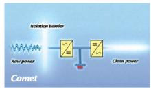
Double conversion topology completely regenerates 100% of the output power from the inverter ensuring that only clean, regulated power is fed to the output. The inverter is an effective isolation barrier against poor power conditions. No raw utility power ever reaches sensitive devices on the output.
