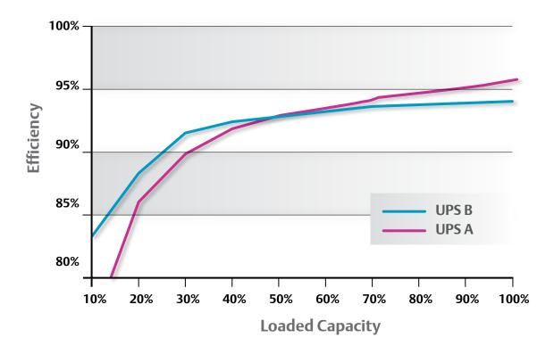
Figure 1. Efficiency curves for two UPS systems are derived by measuring the difference between utility and IT loads from zero to 100 percent capacity.
