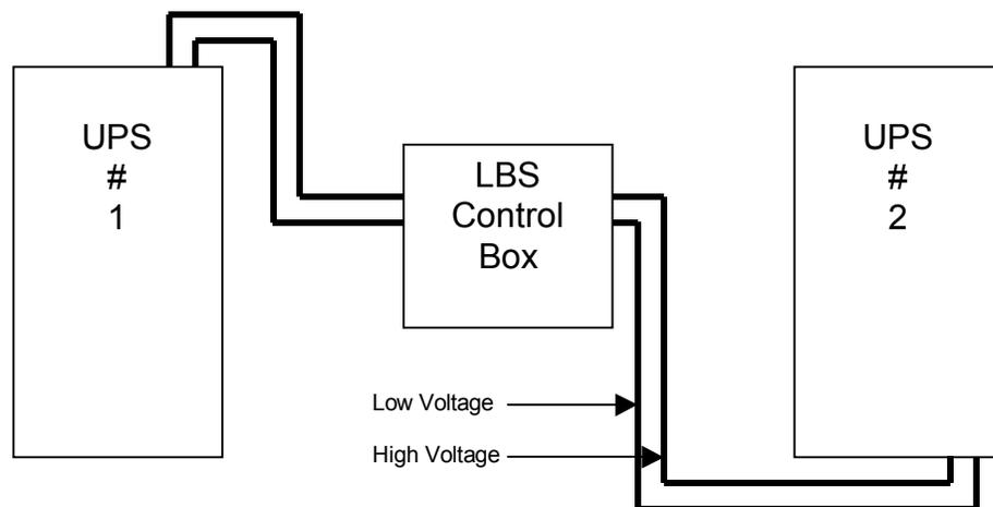
Figure 82 LBS Assembly Diagram
