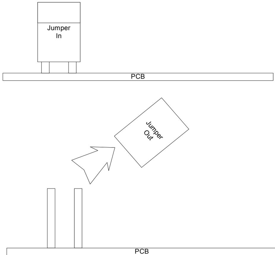
**Figure 9** shows an example of jumper removal. Please consult the documentation with each option to determine the location of the termination resistor jumper.
