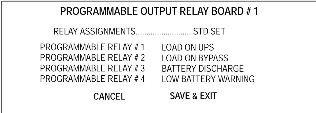
**Figure 27 Programmable Output Relay Board, Std. Set, page 2**
