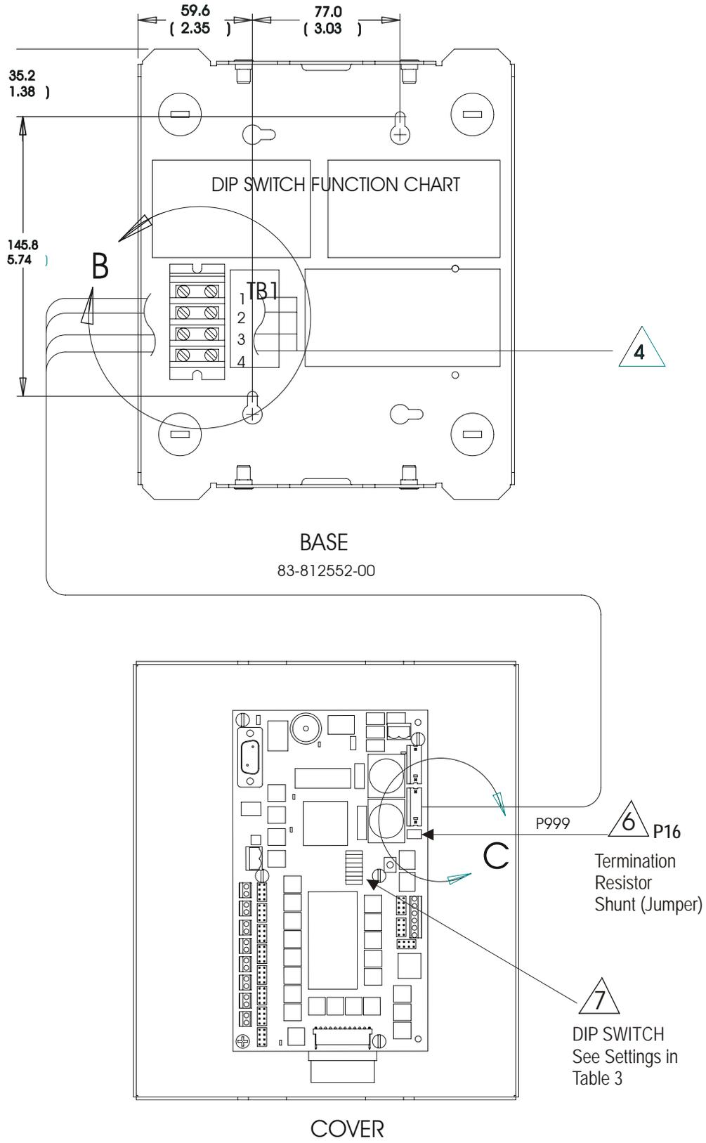
**Figure 41 RAS Details B and C**
