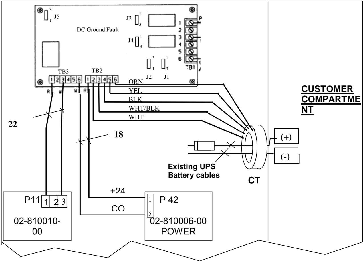
5. Configure the program jumpers on the DC Ground Fault Detector as follows:
