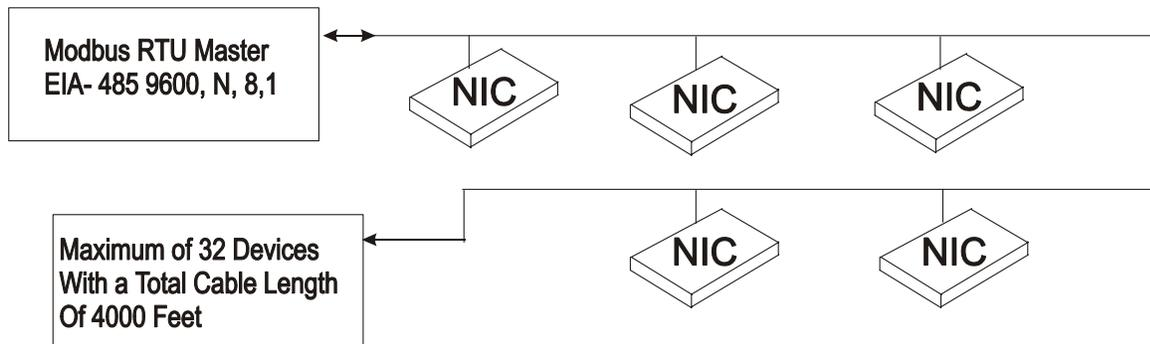
**Figure 73 Installation Exceeding Maximum Specifications**
