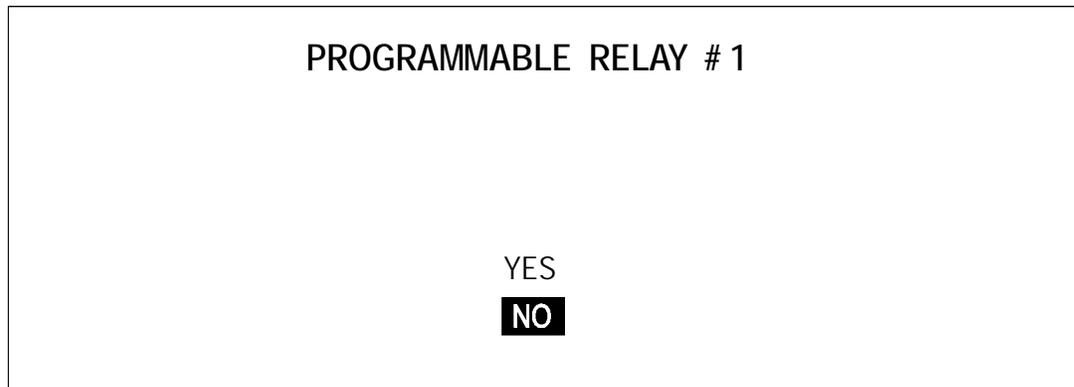
Use the UP and DOWN arrow keys to select YES or NO to enable this option. Once the selection is made Press SELECT. This will return the Operator to the COMMUNICATIONS OPTIONS screen. He may now enable or disable any of the other options he may be installing at this time. When all options to be installed have been enabled; from the COMMUNICATIONS OPTIONS screen select EXIT.
