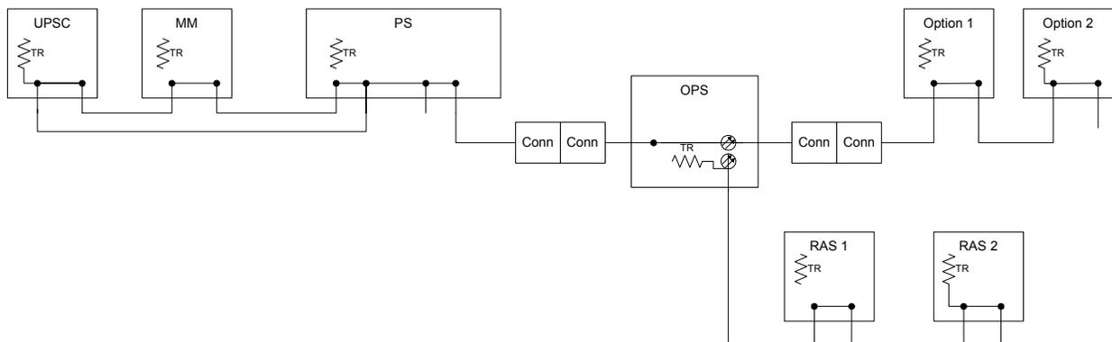
**Figure 7** shows two additional options connected to the CANbus. These options could be an OCDO or an OCDI option. When these options are installed, the termination is enabled on the last unit on the CANbus.
