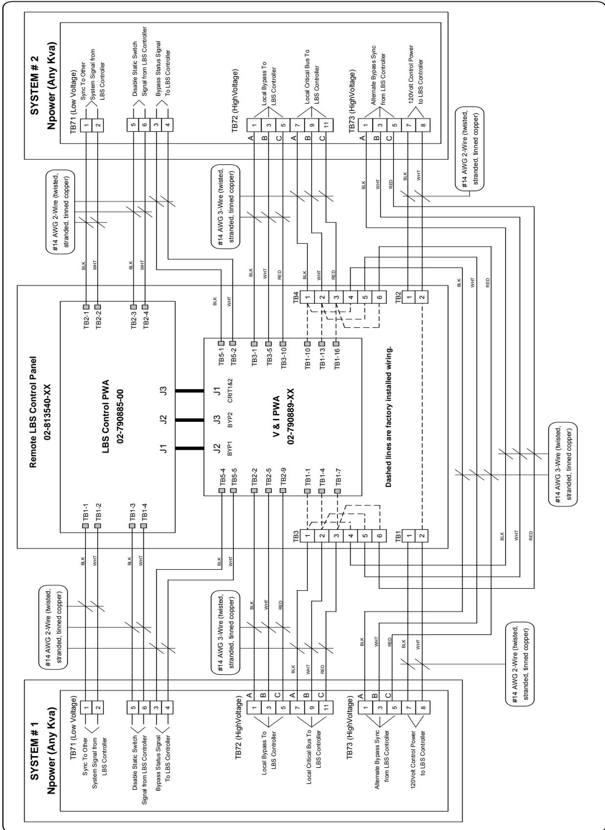
Figure 85 LBS Npower to Npower Wiring with Transformer Cabinet
