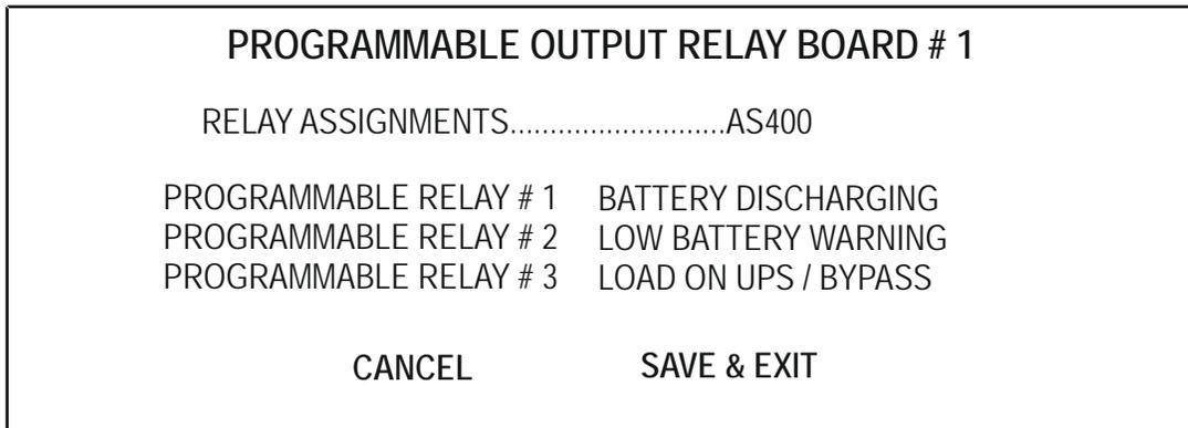
The AS400 pre-assigned relays are shown in this screen.
