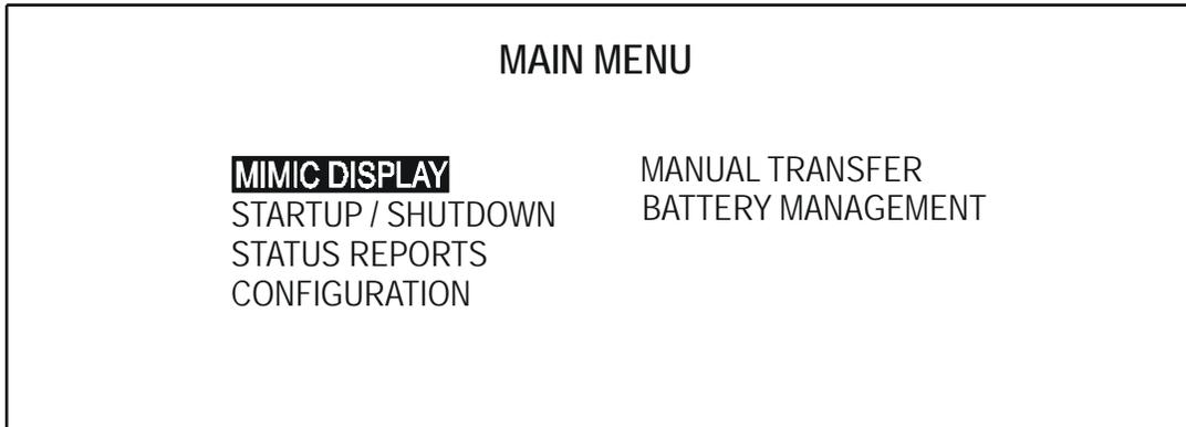
Using the arrow keys move the cursor (reverse video display) to CONFIGURATION. Press SELECT (enter). This will bring up the CONFIGURATION SCREEN shown below
