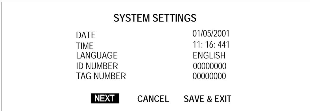
The cursor should have highlighted NEXT, but if it has not, use the arrow keys to highlight NEXT, press SELECT 2 times to scroll through the next setting screens to reach the screen containing the COMM OPTIONS selection as seen below.
