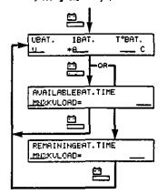
Beattery voltage (VDC), charge (\*) or discharge (-) current (ADC), and battery temperature (decrees Celsus).
