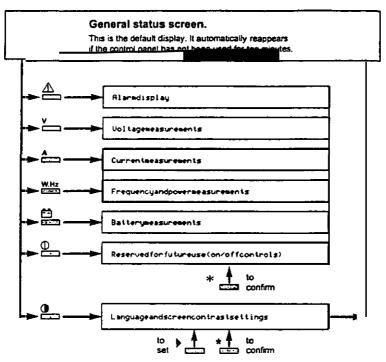
During normal operation. when there are no alarm conditions present and the load is supplied by the UPS inverter output. the display wilt present the general status message:
